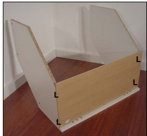
5.1. Secure back panel to top/bottom panels
